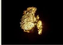
Figure 3a. Images of abaca fibers through scanning electron microscopy 200µm
